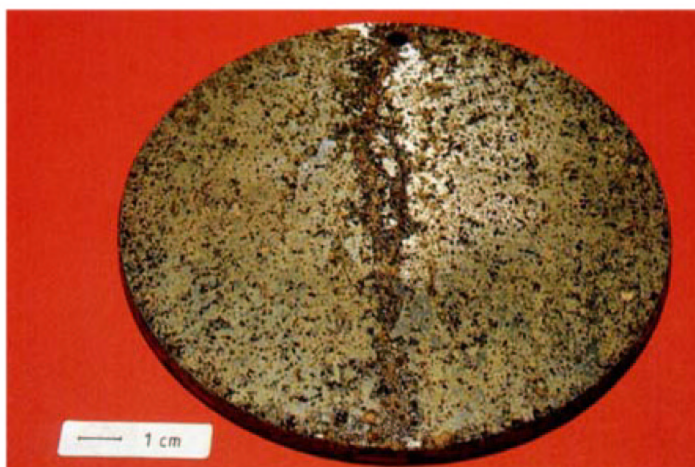
An example of ground ST 35 steel with non-treated surface
