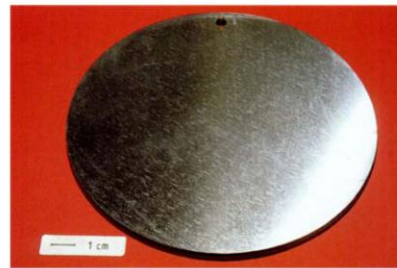
An example of ground ST 35 steel after application of Cylinder Preservation Concentrate VP 130 resp. VP 262
